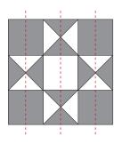
**4.** The Brick border can be moved in all directions by 2" to the next half tile i.e. square or triangle, to accommodate irregular shaped rooms, as long as the overall look is balanced.
