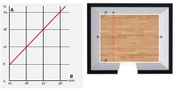
Note that the dimensions of the skirting board must never determine the size of movement joints. With large floor areas, the skirting board must therefore be selected on the basis of the required size for the expansion joint and not vice versa.
