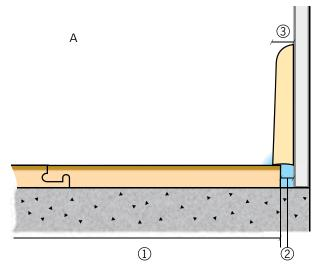
1. Floor width x 1.5 = expansion gap in mm.
