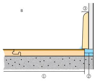
3. Movement joint x 1.5 = skirting board minimum thickness in mm
