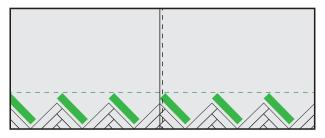
Now install B-planks and cut the most right piece to size.
