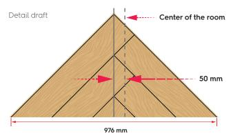
In case you have calculated and built an uneven number of triangles, leave the outer two triangles aside. For the case that you have built an even number of triangles, lay one aside. Lay out the middle triangles with their long side towards the starting wall. Make sure the underlayment is installaed beforehand and the installation line remains visible.
