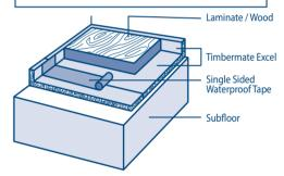
Single sided waterproof tape used in conjunction with the underlay, creates a new, moisture-resistant subfloor onto which the wood or laminate flooring is fitted (in accordance with the manufacturer's recommendations).
